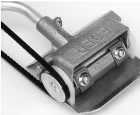
The **EDER Flat Planer EPH-A56** is designed for planing flat or round wood surfaces (from a diameter of 25 cm). The cylinder design achieves high cutting performance with minimum effort. The knives fastened on the rotating cylinder barrel are continuously adjustable. This makes it possible to adjust the cutting radius as well as cutting depth to the desired chip thickness. Four knives are distributed over two levels on the cylinder which create a smooth surface without any vibrations.
