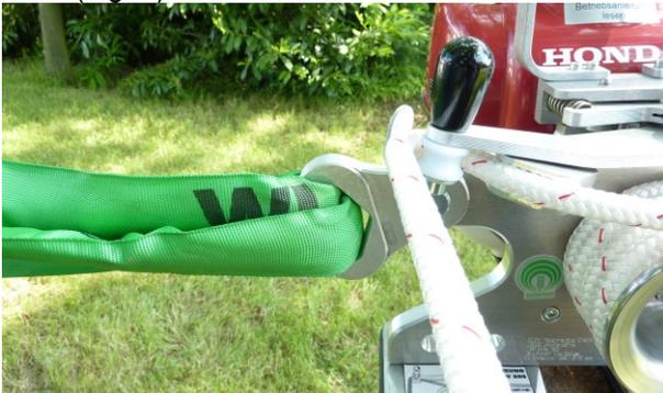
Fig. 20: Guiding the rope through the clamp
