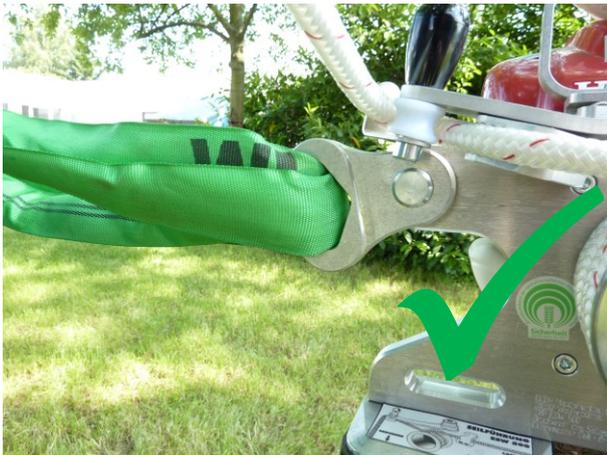
Fig. 22: Correct fastening the EDER Powerwinch 500
