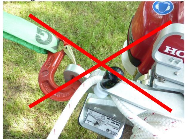
Fig. 21: wrong fastening the EDER Powerwinch 500
