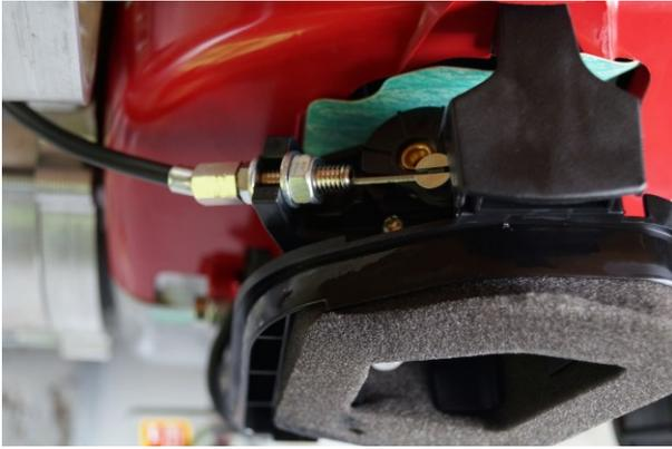
Fig. 27: Adjusting bowdencable
