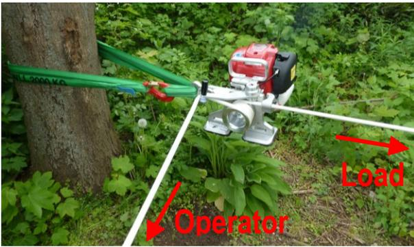
Fig. 19: EDER Powerwinch 500 in working position
