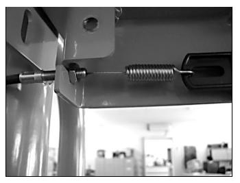
Install the water valve cable spring connector to the water on/off slam latch (5) and anchor the water valve cable (6) to the water control valve housing (8).
