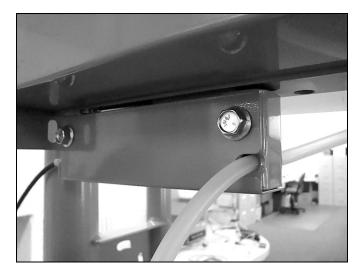
Install the water valve cover (9) and secure it with the 3/8 x 3/4" flanged bolts (4).
