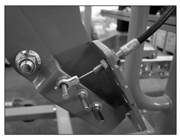
Install the Water line cable (6) to the top stud of the throttle lever assembly. Adjust the nuts to about the mid-point on the threads.
