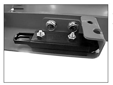
Install the water on/off slam-latch actuator (5) into the water valve bracket (8). Push to the extreme right and secure the water actuator with the #12-24 x 1 1/4" machine screws (2) and nuts (1).
