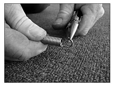
Open the "hook" of the water valve cable spring slightly.
