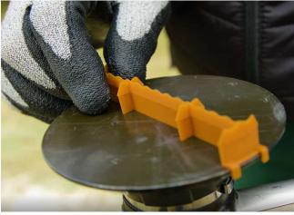
2. The four hooks must snap into place on the impact plate.
