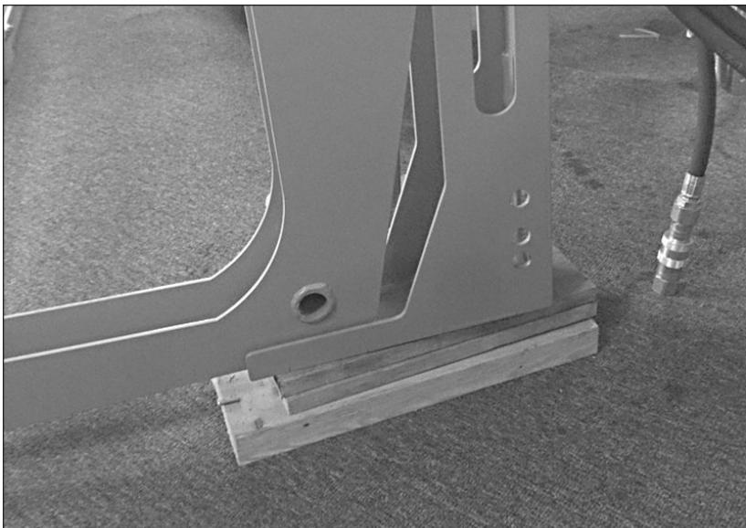
The mounting brackets (item #17) is meant to attach the cradle (item #16) and loader arm (item #15) to the sawmill bed. It is not designed to hold the weight of the log, so it's necessary to firmly support the cradle on the ground. If the ground is uneven and/or soft, use whatever planks or similar necessary to support them properly.
