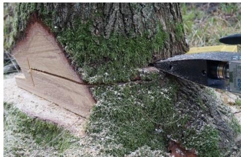
The offset felling cut is obligatory, as it avoids dangerous contact between the Titan 80 Pro and the chainsaw chain.
